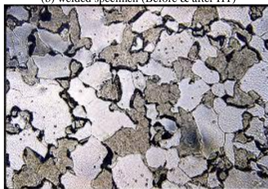
Figure 8: Optical microstructures of heat effected zone after Nital solution etching.
