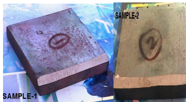
Figure 3: Low alloy steel specimens (without welding) after heat treatment
