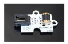
Fig.2.2 Vibration Detection Sensor
