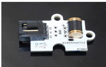
Fig.2.2 Vibration Detection Sensor
