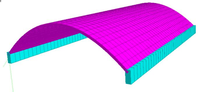
Fig. 4 Model of parabolic cylindrical shell roof
