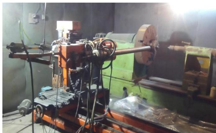
Fig.1 D-Gun Thermal Spray Process Used In the Current Research Work
