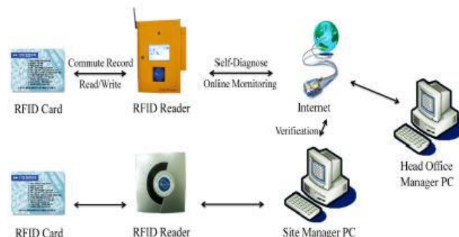
Figure 2.2: RFID communication (Sangyong et al. 2013)
