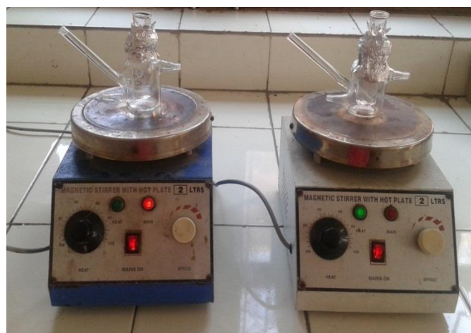
Figure: Franz diffusion cell with skin mounted between compartments.
