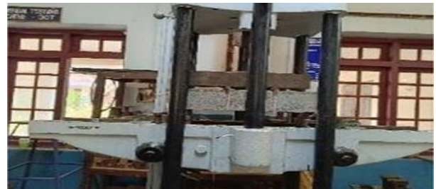
Figure 4 Flexural strength test of concrete beam
